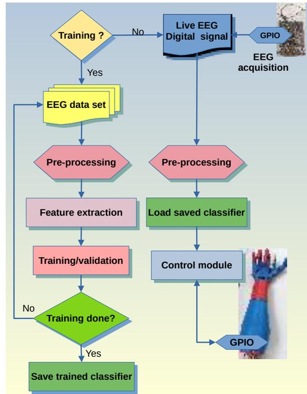
Figure 4: Block diagram of the BCI prosthetic arm control.
