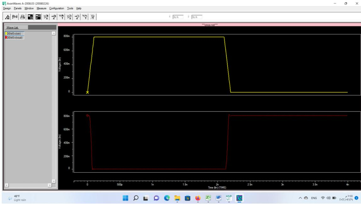
Figure (5). Input / output waveform of the NOT gate circuit
